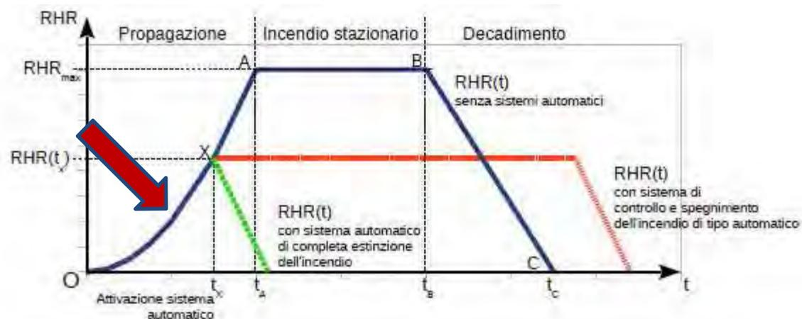
$$RHR(t) = 1000 \left( t/t_\alpha \right)^2 \text{ per } t < t_A$$
